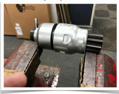
Here, the pin's in place and the drive is ready to slide onto the starter shaft.
